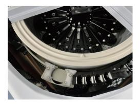
15 reagent positions, supports 4component reagents, with refrigeration function, customization available
