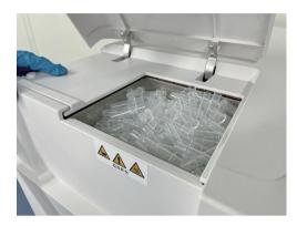
Automatic RV alignment replenishment of 200 at maximum without an interruption in system operation
